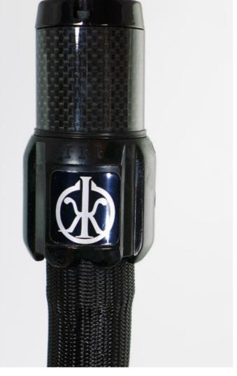
The cable is wider in the middle and stepped down at the ends because the oversize gauge is too thick to fit into the plug housing. (The conductors and shielding are the same throughout the length of the cable: the stepped-down section is only missing the granular mechanical damping/shielding layer.) Cryo-treatment is used wherever possible.
